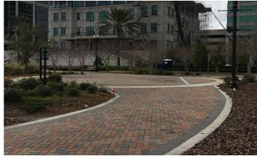
Riverwalk paving should utilize the existing range of paving specified by the city in the City of Jacksonville Riverfront Park Design Criteria, July 2000 Draft. Note: this pattern is intended to be phased
